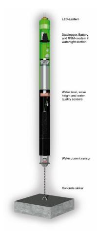
The Smart Buoy with the integrated Oil Spill sensor technology performed successfully in challenging off-shore conditions. As monitoring result, no clear sign of oil contamination was detected. The monitored variation in the collected hydrocarbon concentration was caused by river water originated organic carbon. Nevertheless, as the sensor technology was capable to detect oil contamination in the laboratory experiment, true oil contamination can be detected also in off-shore conditions.
